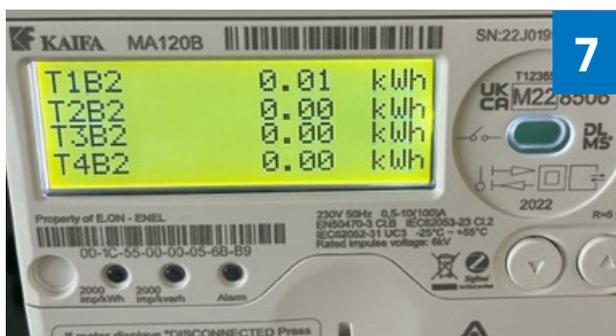
Short press **K1** twice – **T1B2** is the rest of the day KWH – Add together **T1B1** and **T1B2** to get combined day consumption
