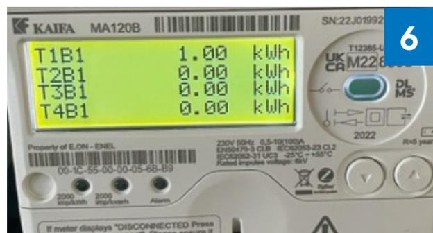
**T1B1** is the total of the 1st KWH of each day charged at the higher rate
