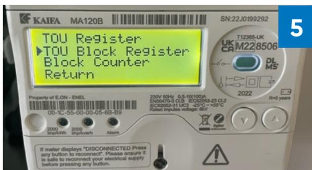
Short press **K1** to move to 'TOU block register' and long press **K2** to enter
